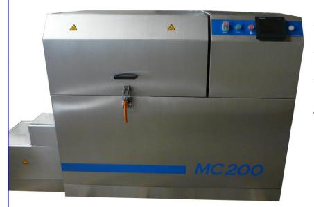
MC200 is based on spray in air technology. Parts are placed into a stainless-steel basket, and submitted to the superior cleaning performance of high flow / low pressure sprayer form 3 Directions while basket rotates. They are perfectly cleaned in just a few minutes.
